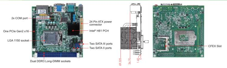
WADE-8016 is based on Intel® H81 chipset and and desktop processor sku like Core™ i7 and i5. WADE-8016 of the Intel® platform will provide high performance and flexibility for functional expansion, such as Gaming, Kiosk, DS, Medical, Defense, Industrial automation and control applications.
