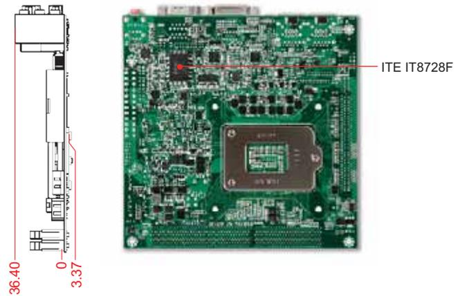
WADE-8014 supports the latest 3<sup>rd</sup> generation Intel® Core™ processor platform in an LGA1155 package, integrated with the memory and PCI Express controller supporting two-channel DDR3 memory and PCI Express 3.0 lanes to provide great graphics performance.
