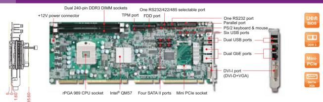
ROBO-8210VG2AR adopts the QM57 chipset and Intel® Core™ i7/i5 and Celeron® processors. Bulit with high performance and lower power consumption than desktop platform, it's suitable for Medical, Industrial Automation and Kiosk applications.
