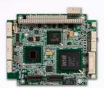
Portwell PEM-P388 is a SUMIT-ISM PC/104 module designed with Intel® Pineview N455 single core 1.66 GHz processor paired with the ICH8M I/O controller hub. Due to low power consumption, high performance and fan less requirement, it is suitable for Automation, Medical, Transportation, Security, Military and HMI applications.
