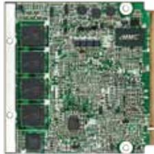
PQ7-M106IE is designed with qualified components for wide-temp support. Hence industrial-grade eMMC storage is adopted to keep system working in -40°C~85°C. In addition, through USB Hub, USB2.0 can be expanded as 6 ports. For Transportation or Outdoor application, PQ7-M106IE will be appropriate solution to meet customer's requirement.
