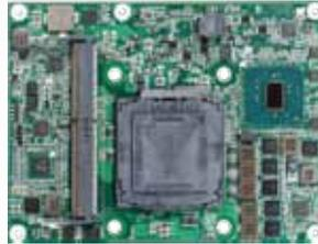
Intel® Skylake-S Core™ i7/i5/i3 processor based on Type VI COM Express module with DDR4 SDRAM, VGA, LVDS, Gigabit Ethernet, SATA 3.0 and USB
