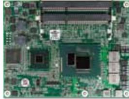
Intel® 5<sup>th</sup> Generation Core™ i7/i5/i3 processor based on Type VI Basic-COM Express 2.0 module with DDR3L ECC SDRAM on Dual SO-DIMM slots, VGA, Display-port, Gigabit Ethernet, SATA and USB
