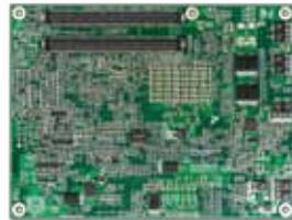
The basic PCOM-B635VG COM Express module supports up to 16GB ECC DDR3L 1333/1600 MT/s SDRAM on two 204-pin SO-DIMM sockets making it faster than its predecessor. Its expansion interface supports one PCI Express x16 Gen3 (8.0GT/s) with three controllers integrated into processor for enhanced video performance and enhance capabilities to be configurable to 2 x8-lane or 1 x8-lane and 2 x4-lane PCI Express ports.
