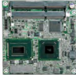
The Portwell PCOM-B219VG is designed with the Intel® QM77 express chipset which offers high computing power with the 3rd generation Intel core family. This provides turbo-boost, vPro, Hyper Threading, 3D Tri-gate Transistors, USB 3.0 and all the other materials necessary of withstanding wide temperature ranges necessary for harsh environment.
