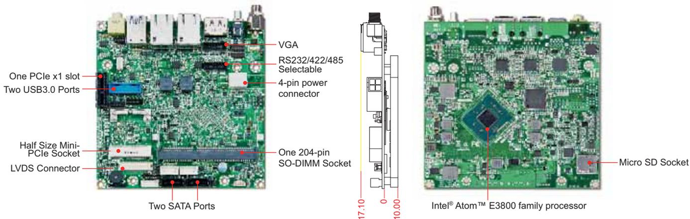
NANO-6060 build with Intel® Atom™ processor E3800 family that not only outputs under 10W for fan-less applications, but also supports a wide industrial temperature from -40°C to 85°C. With its superior up to Quad Core processing power and high capability. Portwell have taken advantage of such technology to furnish a series of products that can meet multiple industrial requirements such as fanless, cost-effective of CPU performance or compact systems..
